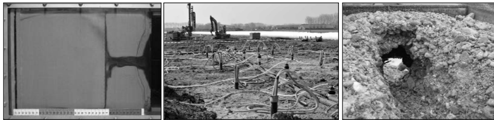
Figure 2 BioGrout research: laboratory testing (left); field testing (centre); prevention of pipe channel growth (right) (FloodProBE, 2012)
